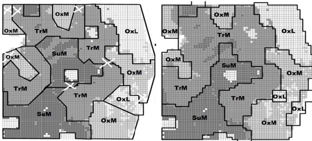
**Figure 5:** This figure compares a set of manually designed dig lines (on the left) to a set of computer generated optimal dig lines (on the right). The grey scale indicates the initial ore type by block grade; black is SuM ; dark grey is TrM; medium grey is OxM; light grey is OxL; and white is waste. The labels on the maps indicate the dig line ore type.
