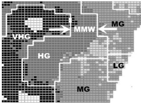
**Figure 2:** An example of an ore control block model. The white lines represent dig lines constrained by a minimum mining width (MMW). The various shades of grey indicate very high grade (VHG), high grade (HG), medium grade (MG), and low grade (LG) ore types.
