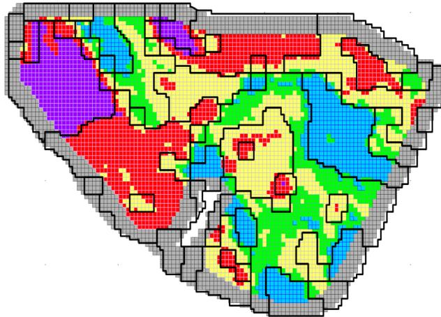
**Figure 2:** Minimum mining width is 4 blocks
