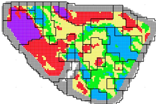
**Figure 3:** Minimum mining width is 6 blocks
