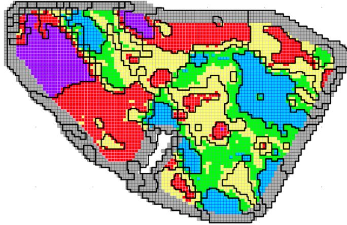
**Figure 1:** Minimum mining width is 2 blocks
